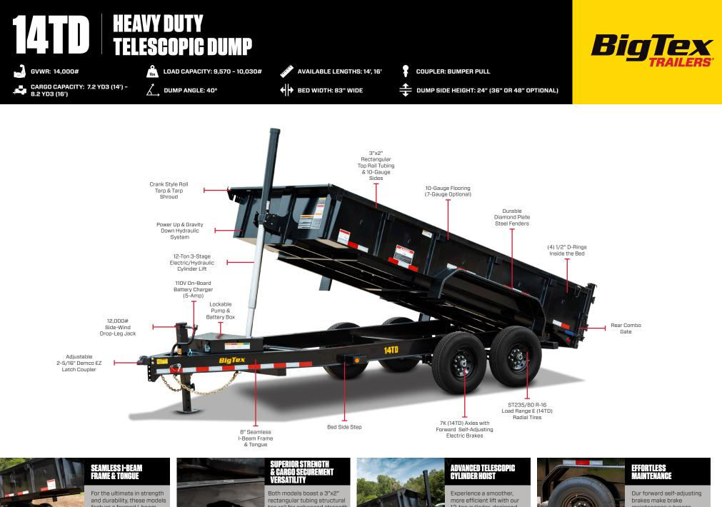
feature a formed I-beam frame with an integral tongue. No cuts. No fishplate. Just a sturdy frame design built to withstand the test of time.
